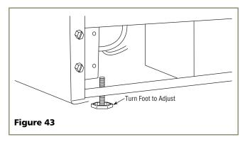
Check the levelness after each adjustment and repeat the previous steps until the unit is level. Go on to 9 Install the Unit.
